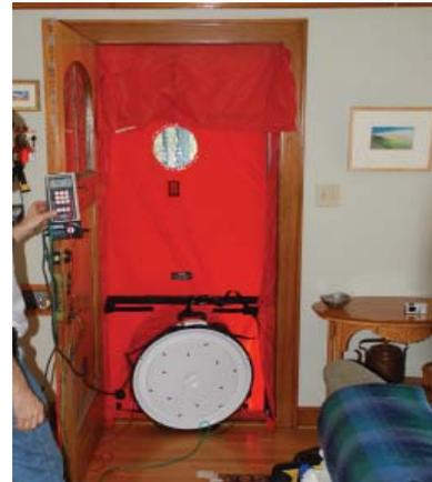
Blower Door Test for Air Leakage
